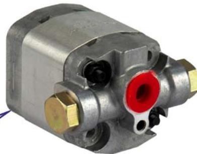
R series: bidirectional pumps with integrated suction check valves and two front outlet ports. They can be fitted on MR type central manifold.
