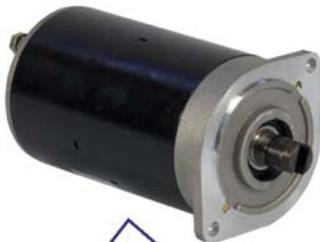
**Frame 80 DC motors:** with or without thermal protector and running time up to 6 min. Power from 0,15kW up to 0,8kW 12 or 24VDC. The permanent magnet construction allow their use in bidirectional units.
